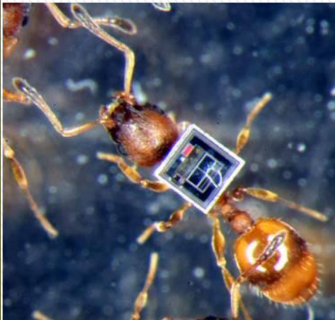
Commercialized IC for specimen tagging purposes [1]
